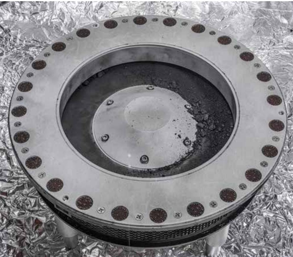
In September, the OSIRIS-REx spacecraft delivered to Earth a capsule of rock and dust from the asteroid Benu. Scientists have started studying debris that adhered to the outside of the collection container (shown).
