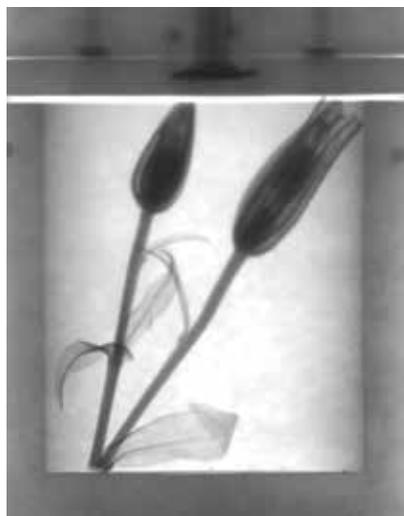
Neutrons suitable for tomography are produced with comparatively massive particle accelerators or as by-products from nuclear reactors. The neutrons are relatively slow moving, with energies one-hundred-millionth those of X-rays in CT scanners. These slow neutrons interact strongly with some low-density materials that X-rays pass through blithely, including lithium, boron and hydrogen.
